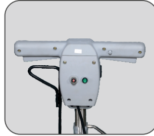
The handle is equipped with safety switches.
