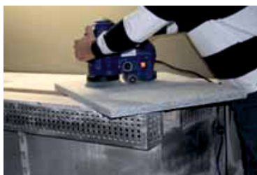
Hard grinding on raw surfaces
